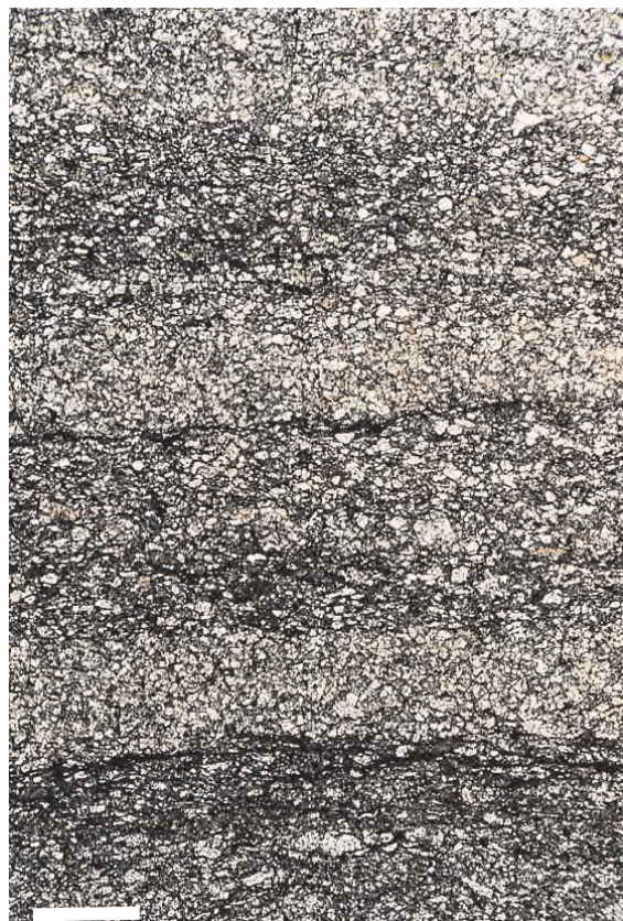
Figure 41: Laminated fine sandstone and siltstone with intercalations of claystone (132a; Gedinnian). Mono- and polycrystalline quartz crystals accompanied by an assemblage of authigenic quartz, muscovite, clay minerals, goethite and hematite. Goethite and hematite are precipitated together with manganese oxides/hydroxides mainly along bedding joints. Length of scale bar is 1 mm.
