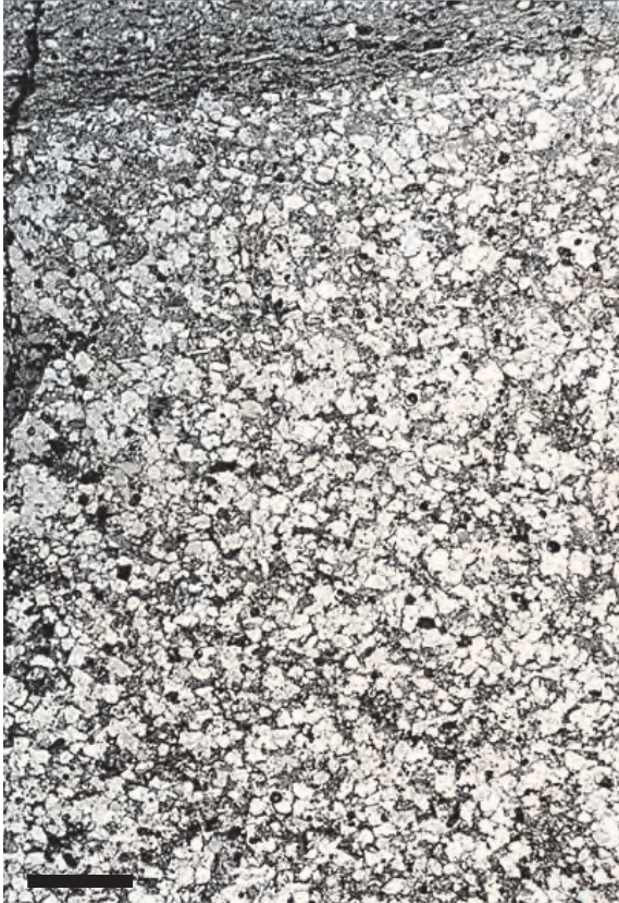
Figure 34: Well sorted fine-grained quartzitic sandstone of Gedinnian age of sample 124 with silt- / clay intercalations in the upper part. Mean grain size of quartz is approx. 0.2 mm. Compared to the other sandstones, a relatively high percentage (about 3%) of fine grained (50-80 \mu ) transparent and opaque heavy minerals such as hematite, rutile, ilmenorutile, titanite occur. The heavy minerals were detected by X-ray diffraction. Length of scale bar is 1 mm.
